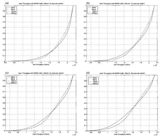
*Figure 1.* User throughput cdf for various loads (WWW traffic, 50 km/h): (a) 8 users per sector; (b) 16 users per sector; (c) 24 users per sector; (d) 36 users per sector.
